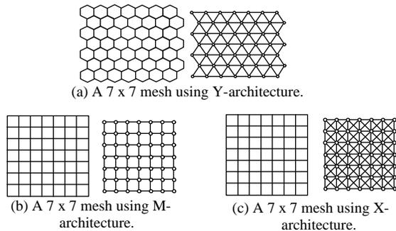
Figure 1:  $7 \times 7$  meshes with different interconnect architectures.
