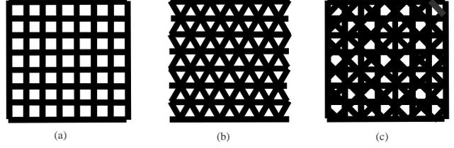
Figure 4: Routing grids in M-, Y- and X-architectures.
