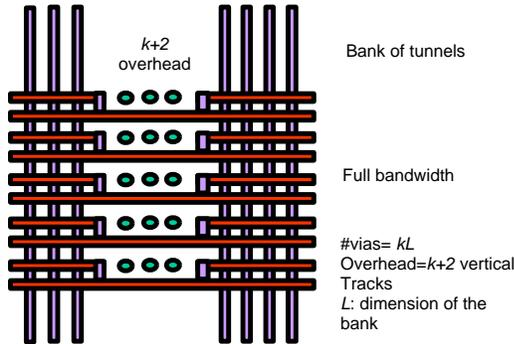
Figure 6: Bank of via tunnels in M-architecture.
